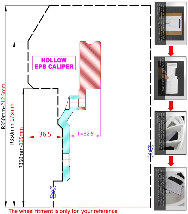
and it can not 100% ensure the clearance between caliper and rim is ok. if there is any interference issue, please change your wheel as possible.
