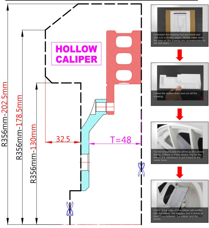
The wheel fitment is only for your reference and it can not 100% ensure the clearance between caliper and rim is ok. if there is any interference issue, please change your wheel as possible.
