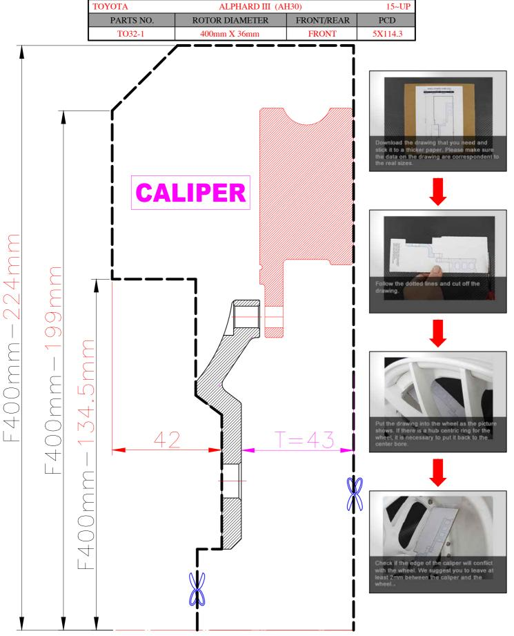
The wheel fitment is only for your reference and it can not 100% ensure the clearance between caliper and rim is ok. if there is any interference issue, please change your wheel as possible.
