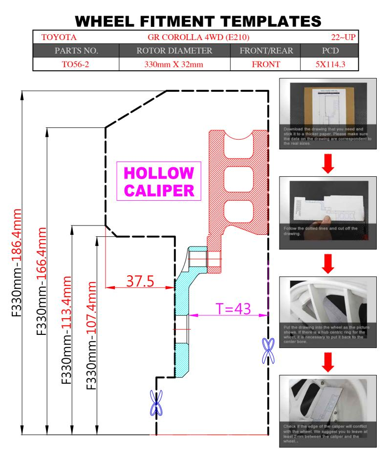
The wheel fitment is only for your reference and it can not 100% ensure the clearance between caliper and rim is ok. if there is any interference issue, please change your wheel as possible.
