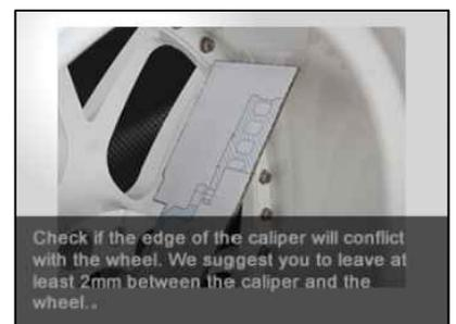
The wheel fitment is only for your reference and it can not 100% ensure the clearance between caliper and rim is ok. if there is any interference issue, please change your wheel as possible.
