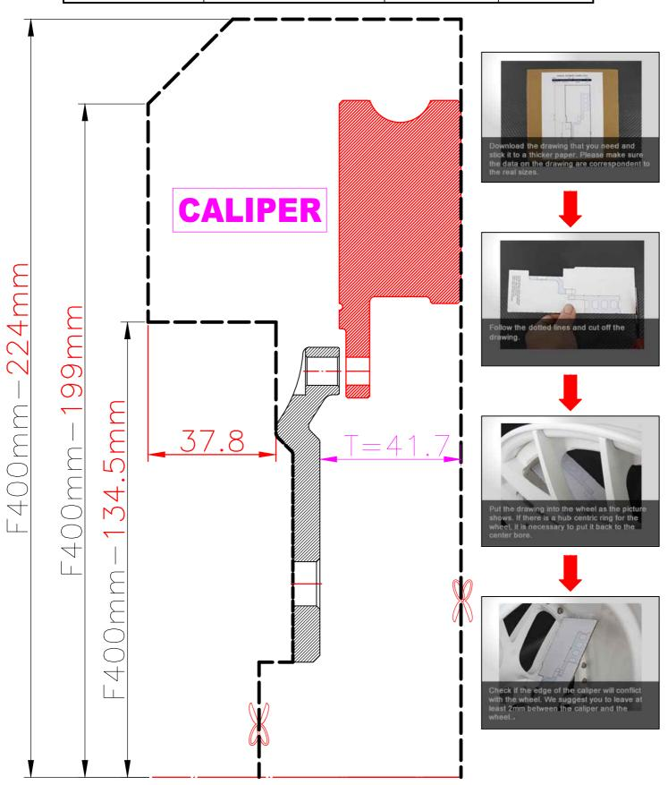
The wheel fitment is only for your reference and it can not 100% ensure the clearance between caliper and rim is ok.
