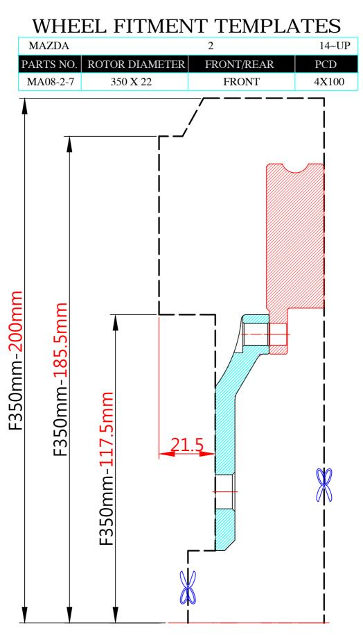
The wheel fitment is only for your reference and it can not 100% ensure the clearance between caliper and rim is ok. if there is any interference issue, please change your wheel as possible.
