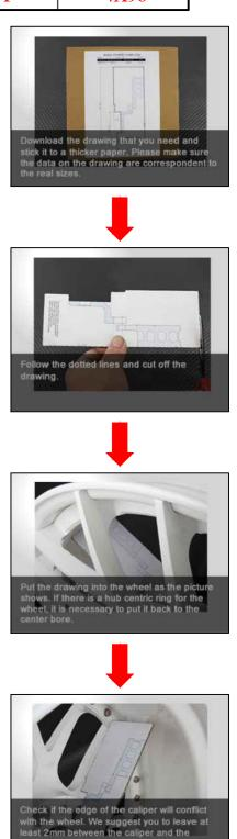
The wheel fitment is only for your reference and it can not 100% ensure the clearance between caliper and rim is ok. if there is any interference issue, please change your wheel as possible.
