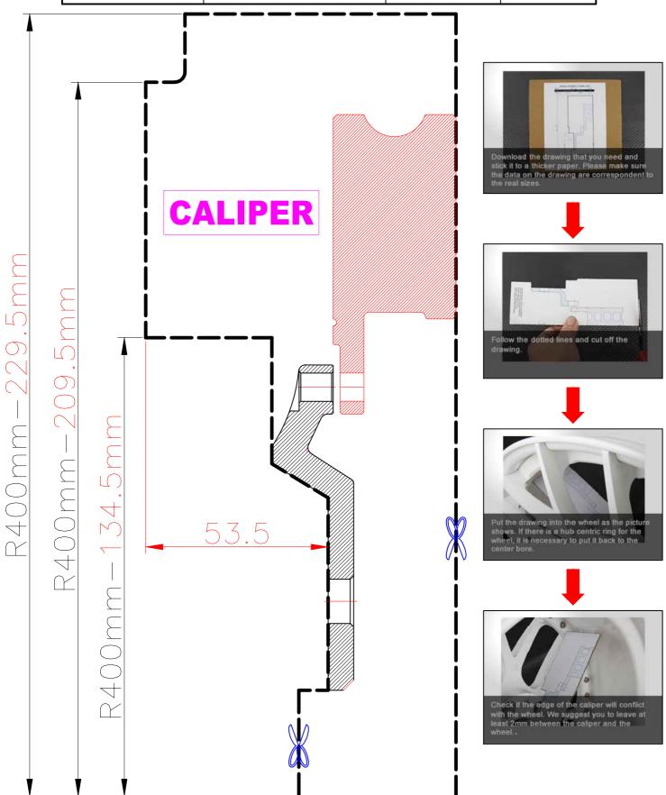
The wheel fitment is only for your reference and it can not 100% ensure the clearance between caliper and rim is ok.
