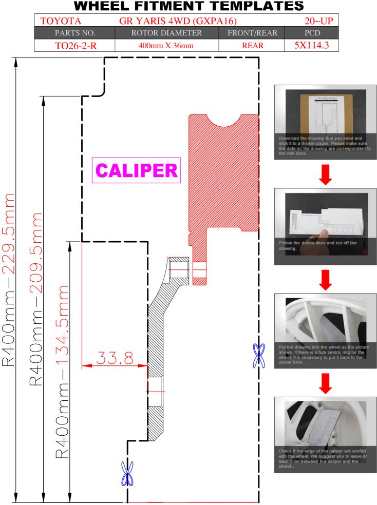
The wheel fitment is only for your reference and it can not 100% ensure the clearance between caliper and rim is ok.
